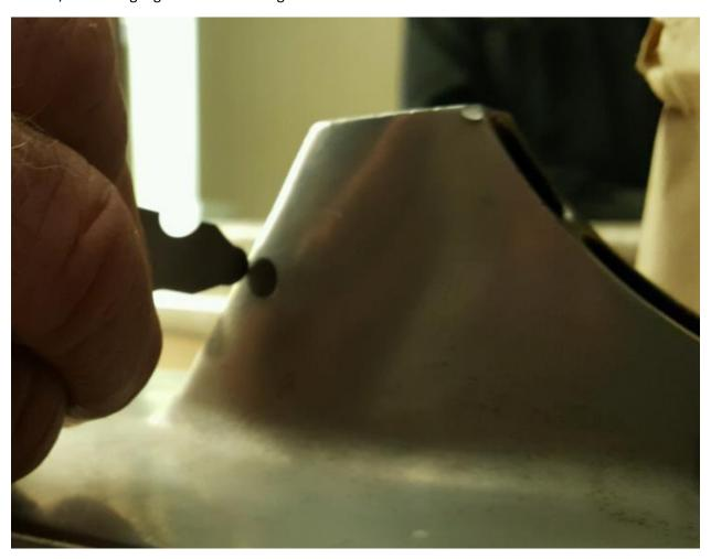
Use a small hole gauge to measure the inlet diameter
