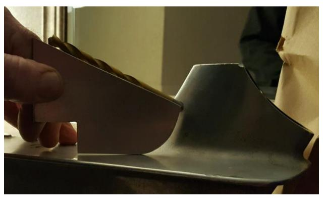
Also use the template to check the height of the center of the inlet hole
