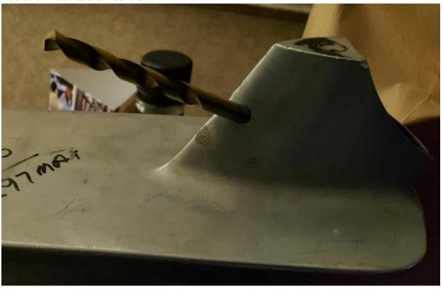
Use the template to check the angle of the inlet hole. The template is only a guide to assist you.
