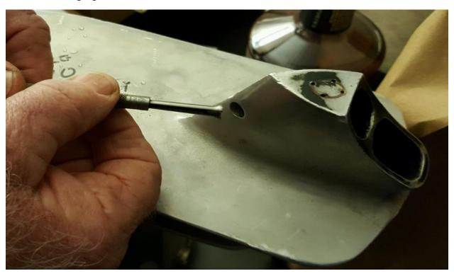
Insert a drill bit into the inlet hole
