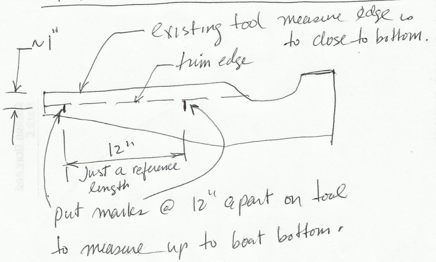
Then with tool in place adjust engine tilt and measure from tool edge at marks up to bottom. To be level both measure the same.
